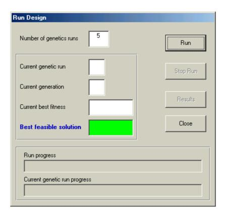
While the design process is on, the progress bars on the bottom of the dialogue show its progress.
